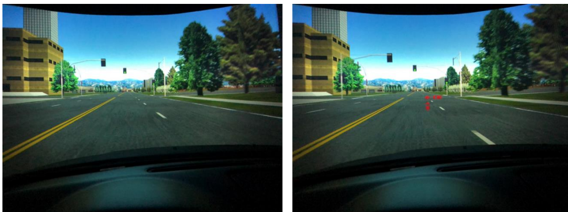
16 Figure 2 – No alert displayed (left) versus alert displayed (right) as a HUD
