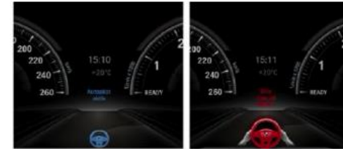
Automation available (left) and request-to-intervene (right): (Jarosch et al, 2019)
