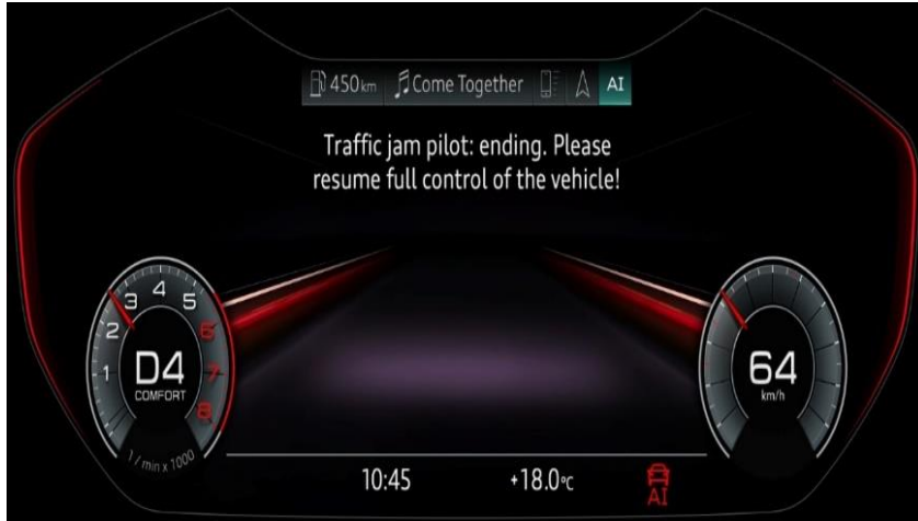
TOR interface when the traffic jam pilot of Audi A8 request drivers to take back control ( source: AUDI AG, Image No: A1710305 )
