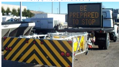
b. Extended duration vehicle with truck-mounted attenuator (with traffic flow) Source: Tennessee DOT
