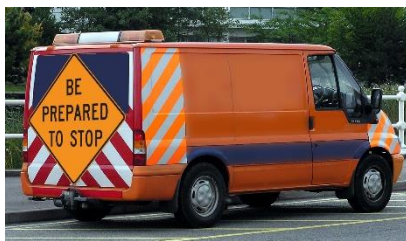
a. Quick response vehicle (with traffic flow) (Photo simulation)
